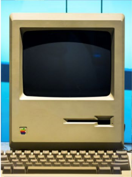
Macintosh, Apple, US, 1984 The innovative Macintosh — Apple's second attempt at a 128K-based personal computer. Following the failure of the Lisa — was a small, self-contained personal computer with a user-friendly, window-like graphical desktop. Graphical designers, artists, and educators
