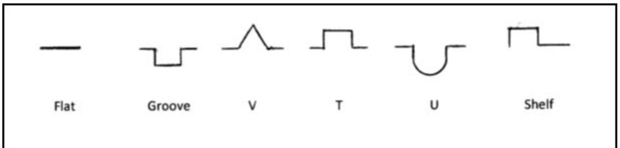
FIGURE 9: STANDARD BEVEL PROFILES
